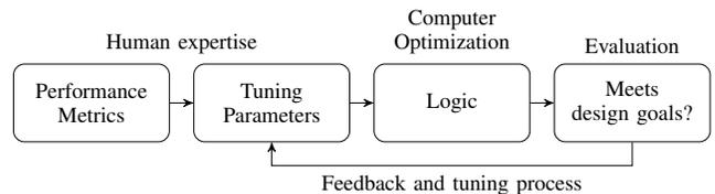
Figure 2: ACAS X logic tuning process.
