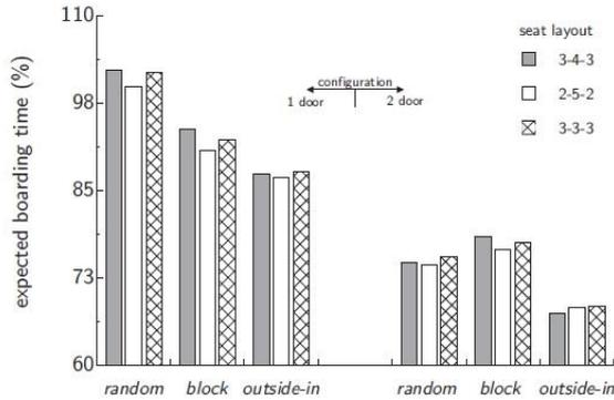
Figure 12. Boarding efficiency using Boeing B777-200 considering random, outside-in, and block strategies, as well as 3 seat (3-3-3, 3-4-3, 2-5-2) and door configurations (1, 2) at standard values for CR = 85%, SLF = 85%, AR = 28 passengers per minute, using random strategy and 2-5-2 seat layout as reference.
