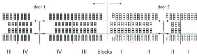
Figure 16. A380 seat layouts with 8 blocks for the two door configuration.
