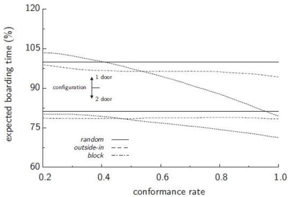
Figure 17. A380. Three boarding sequences (*random*, *outside-in*, *block*), 1 and 2 door configuration at AR = 28 passenger per minute and SLF = 0.85.
