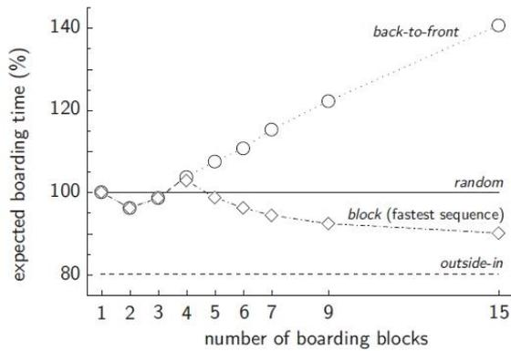
Figure 6. Efficiency of block strategies using different block numbers
