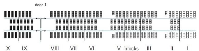
Figure 15. A380 seat layouts with 10 blocks for the one door configuration
