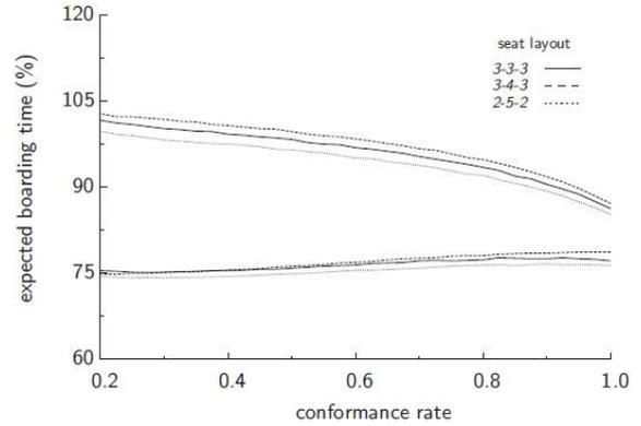
Figure 14. Boarding time using Boeing B777-200, block sequence, 3 seat configurations, 1 and 2 door
