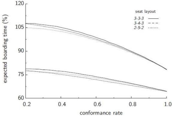
Figure 13. Boarding time using Boeing B777-200, outside-in sequence, 3 seat configuration, 1 and 2 door
