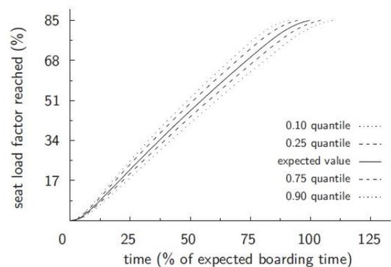
Figure 5. Boarding progress using the default boarding parameters
