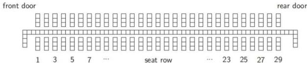
Figure 2. Grid based simulation environment for an Airbus A320 seat layout
