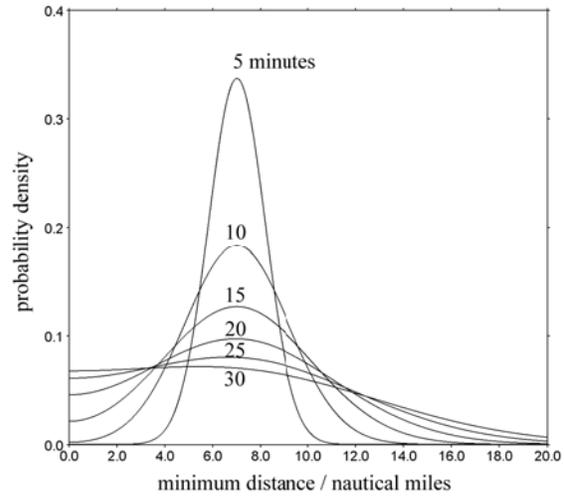
**Figure 15 Minimum distance probability density functions (predicted minimum distance = 7 nautical miles)**
