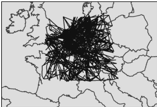
**Figure 1. Flight routes included in the air traffic sample for the European 5 states region.**
