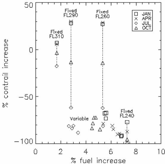
**Figure 6. Contrail increase against fuel increase for each of the combinations of altitude restrictions. For the fixed altitude restrictions, the contrail change shown for each month is averaged over the 5 years.**
