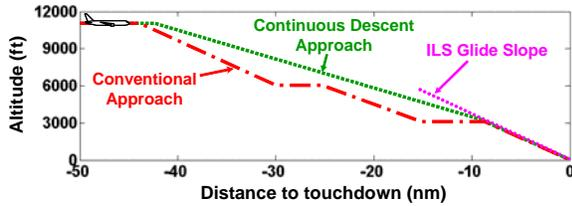
**Figure 1: Conventional vs. Continuous Descent Approach Procedures.**
