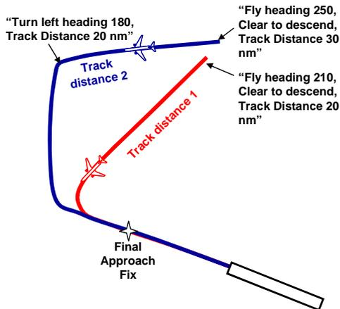
**Figure 2: Lateral View of Basic CDA Concept.**
