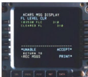
**Figure 1. CPDLC Display for Pilots**
