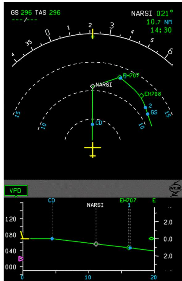
Figure 10: ND with flap/gear deployment cues and vertical view
