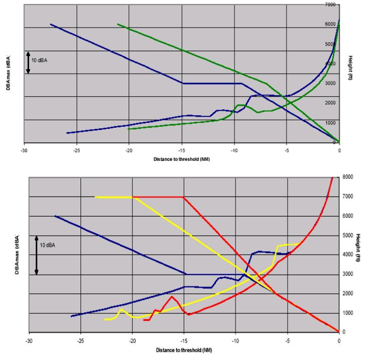
Figure 3: Vertical profile and maximum noise level for the procedure I (reference approach, blue), procedure III (green), procedure IV (red) and V (yellow).
